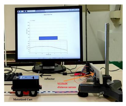
Experimental setup with the VL53L0X Distance Sensor to visualise and record the positiontime graphs of a Variable Speed Motorized Cart with three-stage switch for forward, off, and
