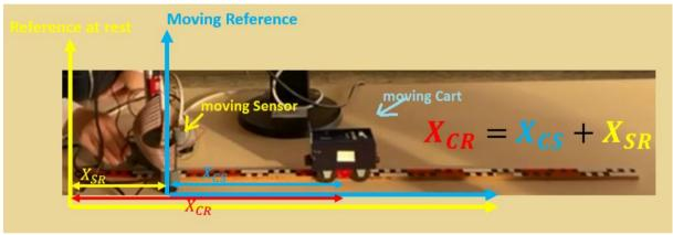
Experimental setup with the VL53L0X Distance Sensor to visualise and record the relative position-time graphs of a Cart to the Motion Sensor as they move in opposite directions towards each other, in opposite directions away from each other, and in the same direction.
