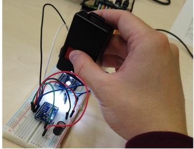
A step voltage pulse is generated at two pins of the Raspberry Pi by a light-dependent resistor (LDR) operated switch. Through the covering/uncovering of the LDR, the input signal at the GPIO-Pin-IN of the Raspberry Pi changes back and forth from a constant positive value to zero volts causing the charging and discharging of the
