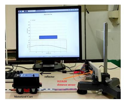
Experimental setup with the VL53L0X Distance Sensor to visualise and record the positiontime graphs of a Variable Speed Motorized Cart with three-stage switch for forward, off, and
