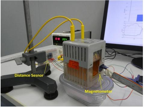
Magnetic flux density against position along the axis of a coil recorded with the MLX90393 triple-axis magnetic sensor and the VL53L0X Motion Sensor.
