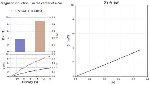
Various graphical representations on the PhyPiDAQ-window as measuring the magnetic flux density at the centre of a coil carrying a linear increasing current.
